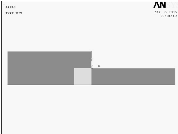
Figure 3.47 Two rectangular areas of different sizes to be added to create a stepped beam area.
