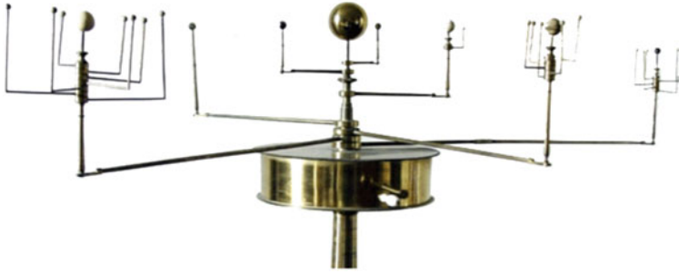
Fig. 4.11 In this mechanical orrery by Gilkerson, housed in the Armagh Observatory the movement of the planets and their moons are mechanically simulated. It is not possible to access an arbitrary position of the system without moving through intermediate states. This is a feature of simulation systems: they do not have a closed form or analytic solution. To compute the state of the system at t_{12} one must determine the state at t_{11} and move from there
