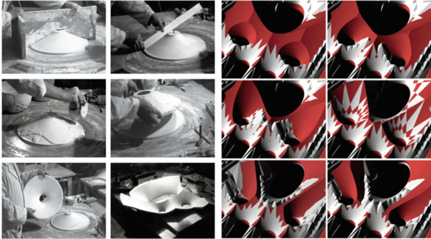
Fig. 14.4 Finding points of intersection on Gaudí's clerestory window. To the left , plaster makers using traditional techniques (Burry 2011b © Mark Burry); to the right , overlaying the digitised plaster models with variable hyperboloids of revolution allowed the team to find the best fit (Burry 2011b © Mark Burry)
