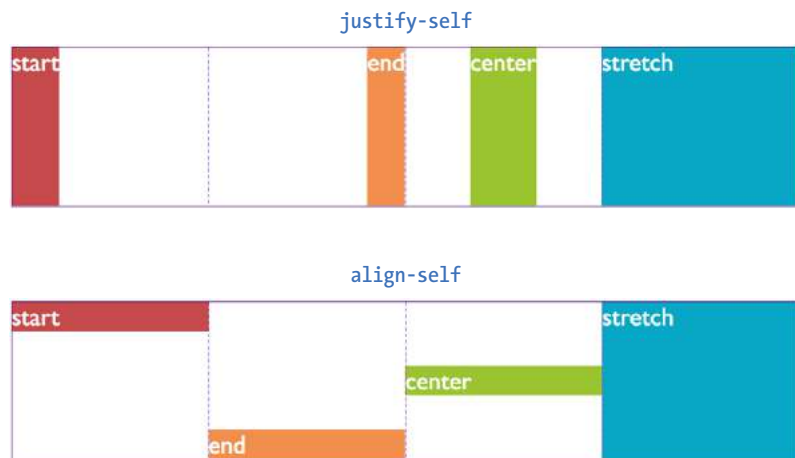
FIGURE 16-45. Values for justify-self and align-self for aligning a grid item within its respective grid area. These values have the same use in the justify-items and align-items properties that are used to align all the items in the grid.
