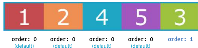
FIGURE 16-22. Changing the order of items with the order property. Setting box3 to order: 1 makes it display after the rest.
