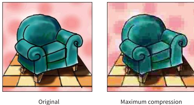
FIGURE 23-3. JPEG compression discards image detail to achieve smaller file sizes. At high compression rates, image quality suffers, as shown in the image on the right.
