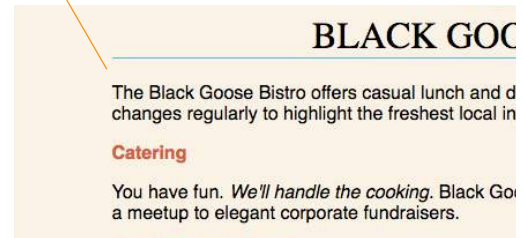
FIGURE 4-18. A missing end bracket makes the browser think the following characters are part of the tag, and therefore the headline text doesn't display.
