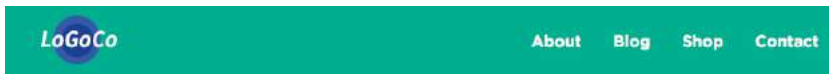
FIGURE 16-13. Using a margin to adjust the space around flex items. In this example, the right margin of the logo item pushes the remaining items to the right.
