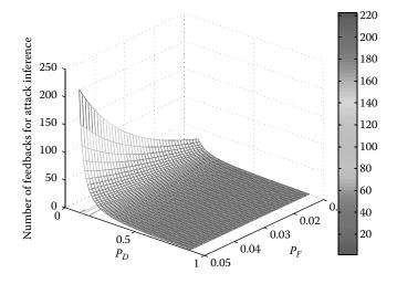
Figure 2.5: Expected number of feedbacks required for the sequential defense scheme to detect a degree attack. The critical values for the WWW, the Internet, and the EU power grid to break down are 21,824, 187, and 766, respectively.
