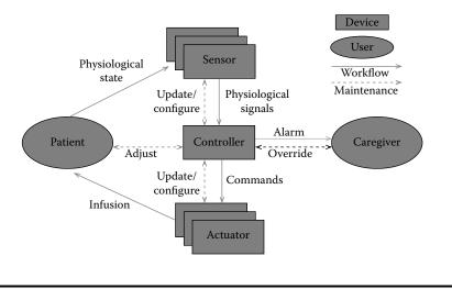
Figure 13.7: MCPS control loop.
