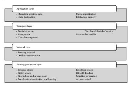
Figure 1.4: Possible attacks based on architecture.
