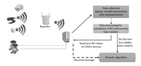
Figure 17.3: Principle scheme of cognitive security work in the capillary network. BO, backoff time; CSMA, carrier sense multiple access.
