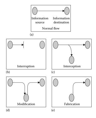
Figure 10.1: Principal attack vectors in IoT device communication.
