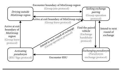
Figure 8.7: State diagram of vehicles.
