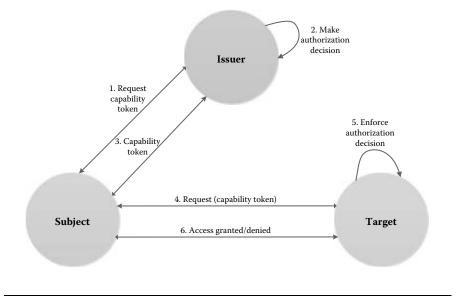
Figure 18.5: Authorization process based on DCapBAC.
