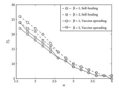
Figure 4.14: Optimal control signal distribution time via dynamic programming under different ( $\alpha$ ,  $\beta$ ) configurations in IoT networks. N = 2000, L = 50,  $I_0 = 1/N$ ,  $\delta = 1.1$ ,  $\lambda_{inf} = \lambda_{pro} = 0.05$ ,  $\eta_{inf} = 6$ ,  $\eta_{pro} = 3$ ,  $\kappa = 0.1$ ,  $T_f = 200$ , M = 1000, t' = 1, and  $c = 10^{-3}$ .
