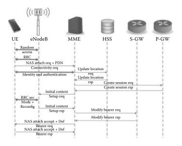
Figure 20.2: NAS attach signaling procedure.
