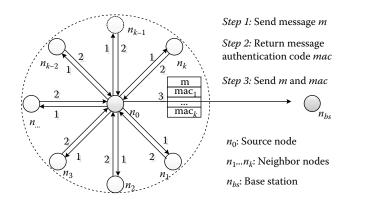
Figure 12.1: Basic network model of cooperative authentication.
