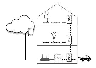
Figure 5.1: A sample digitalSTROM SHS.
