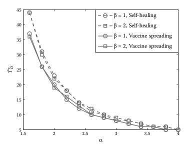
Figure 4.15: Optimal control signal distribution time via early-stage analysis under different ( $\alpha$ ,  $\beta$ ) configurations in IoT networks. N = 2000, L = 50,  $I_0 = 1/N$ ,  $\delta = 1.1$ ,  $\lambda_{inf} = \lambda_{pro} = 0.05$ ,  $\eta_{inf} = 6$ ,  $\eta_{pro} = 3$ ,  $\kappa = 0.1$ ,  $T_f = 200$ , t' = 1, and  $c = 10^{-3}$ .
