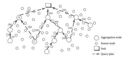
Figure 16.4: A sensor network with a DAG-structured query plan.
