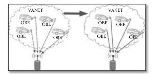
Figure 13.5: Architecture of VANET content delivery.
