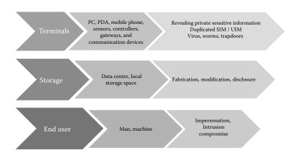
Figure 1.8: Possible attacks based on components.
