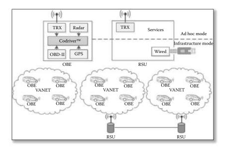
Figure 13.1: Network architecture of VANET.
