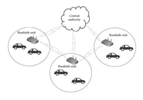
Figure 3.1: Architecture of vehicular ad hoc network
