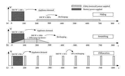
Figure 7.12: Examples of load shaping strategies. (From G. Kalogridis et al. Privacy for smart meters: towards undetectable appliance load signatures. In *Smart Grid Communications (SmartGridComm)*, 2010 First IEEE International Conference on.)
