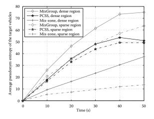
Figure 8.11: Performance comparison of actual pseudonym entropy of a target vehicle.
