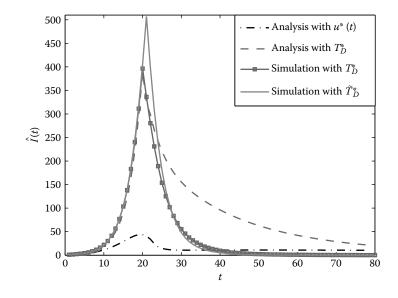
Figure 4.12: Infected population under self-healing scheme in IoT networks. N = 2000, L = 50,  $I_0 = 1/N$ ,  $\delta = 1.1$ ,  $\lambda_{inf} = \lambda_{pro} = 0.05$ ,  $\eta_d = 6$ ,  $\eta_{pro} = 3$ ,  $\alpha = 2$ ,  $\beta = 1$ ,  $\kappa = 0$ ,  $T_f = 200$ , M = 1000,  $\Lambda_I(0) = 200$ ,  $\Lambda_R(0) = 100$ , t' = 1, and  $c = 10^{-3}$  over 300 simulations.
