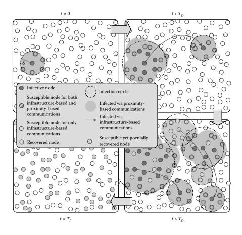
Figure 4.11: Illustration of malware propagation and control signal distribution in IoT networks. Proximity-based and infrastructure-based communication links are exploited for malware propagation. A node is infected at t = 0.  $T_D$  denotes the control signal distribution time, and  $T_f$  denotes the time instance for the eradication of the epidemic.
