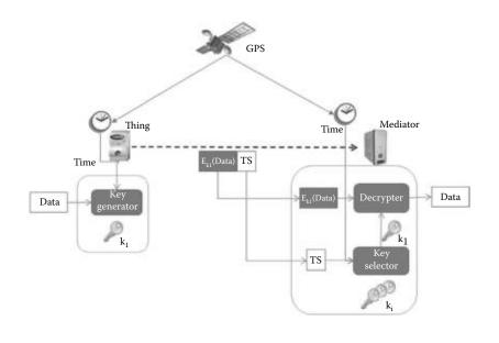
Figure 17.1: Principle of time-based secure key generation.
