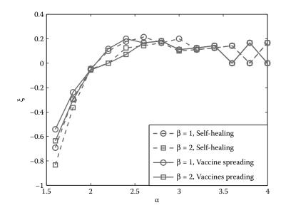
Figure 4.16: Relative difference of optimal control signal distribution time under different ( $\alpha$ ,  $\beta$ ) configurations in IoT networks. N = 2000, L = 50,  $I_0 = 1/N$ ,  $\delta = 1.1$ ,  $\lambda_{inf} = \lambda_{pro} = 0.05$ ,  $\eta_{inf} = 6$ ,  $\eta_{pro} = 3$ ,  $\kappa = 0.1$ ,  $T_f = 200$ , M = 1000, t' = 1, and  $c = 10^{-3}$ .
