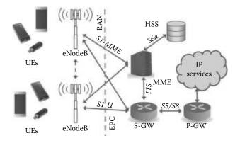
Figure 20.1: LTE network architecture.
