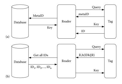
Figure 7.6: (a) Hash locking: a reader unlocking a hash-locked tag; (b) randomized hash locking: a reader unlocks a tag whose ID is *k* in the randomized hash-lock scheme. (Redrawn from S.A. Weis et al. in D. Hutter et al. [eds]. *Security in Pervasive Computing*, Springer, Berlin, 2004.)
