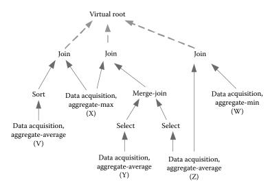
Figure 16.3: DAG-structured query plan.
