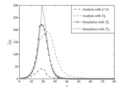
Figure 4.13: Infected population under vaccine-spreading scheme in IoT networks.  $N = 2000, L = 50, I_0 = 1/N, \delta = 1.1, \lambda_{inf} = \lambda_{pro} = 0.05, \eta_{inf} = 6, \eta_{pro} = 3, \alpha = 2, \beta = 1, \kappa = 0.1, T_f = 200, M = 1000, \Lambda_I(0) = 200, \Lambda_R(0) = 100, t' = 1, and c = 10^{-3}$  over 300 simulations.
