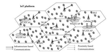
Figure 4.1: IoT platform with infrastructure-based and proximity-based communications.
