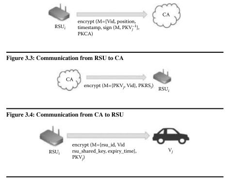
Figure 3.5: Communication from RSU to vehicle
