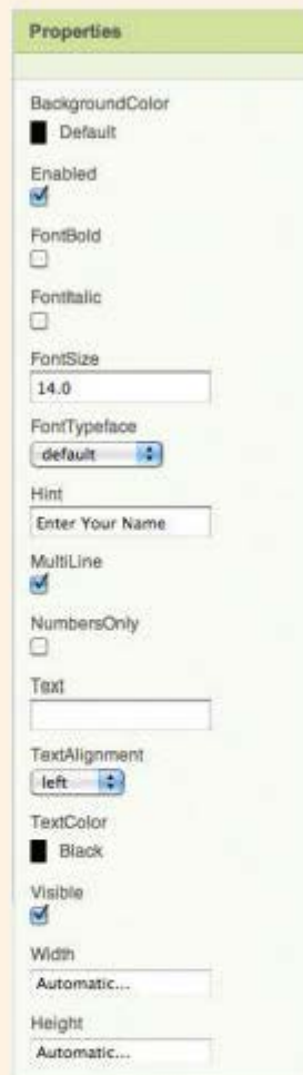
Figure 4-5 Setting the Hint property for a TextBox component
