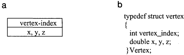
FIGURE 19 Vertex entity description: (a) Storage allocation and (b) C declaration.
