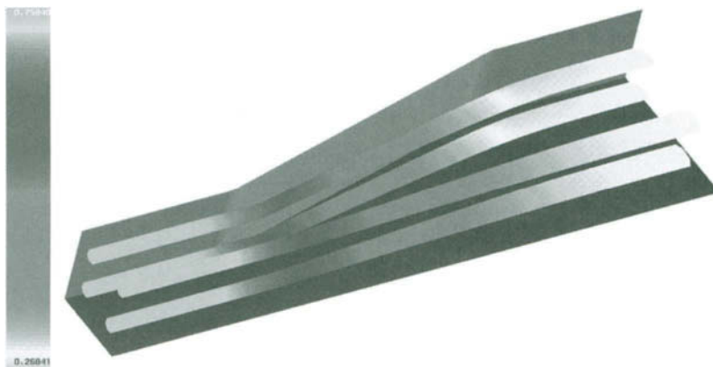
FIGURE 11 Four streamtubes in a rectangular duct where color and radius indicate the flow velocity and pressure, respectively. Reprinted from S. Park and K. Lee, (1997) with permission from Elsevier Science.
