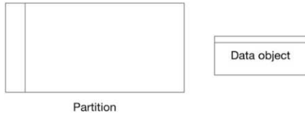
Figure 3.16: Notation elements to represent responsibilities and data flows in activity diagrams
